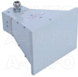
LB-20200-NFSPPO Broadband Horn Antenna 2-20GHz 12dB Gain N Type Female
