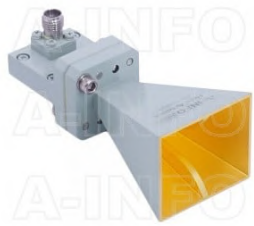
LB-180400-KF Broadband Horn Antenna 18-40GHz 15dB Gain 2.92mm Female
