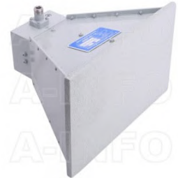
LB-10180-NFSPS Broadband Horn Antenna 1-18GHz 11dB Gain N Type Female
