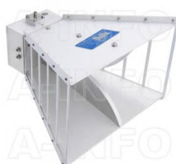
LB-8180-SF Broadband Horn Antenna 0.8-18GHz 12dB Gain SMA Female
