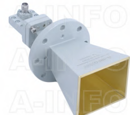
LB-180400H-KF Broadband Horn Antenna 18-40GHz 20dB Gain 2.92mm Female
