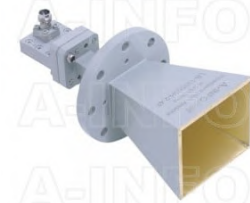
LB-180500H-2.4F Broadband Horn Antenna 18-50GHz 20dB Gain 2.4mm Female
