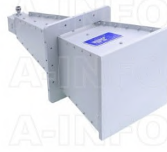
LB-20180H-NFSP0 Broadband Horn Antenna 2-18GHz 17dB Gain N Type Female
