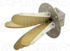
LB-OSJ-20180-SF Open Boundary Quad-Ridged Dual Polarization Horn Antenna 2-18GHz 13dB Gain SMA Female
