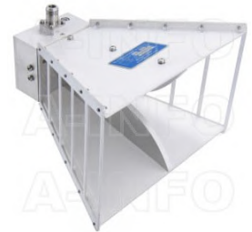
LB-8180-NF Broadband Horn Antenna 0.8-18GHz 12dB Gain N Type Female
