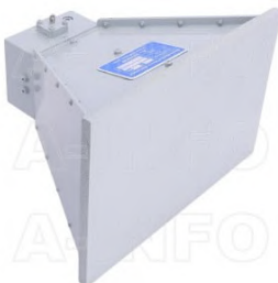
LB-10180-SFSP0 Broadband Horn Antenna 1-18GHz 11dB Gain SMA Female
