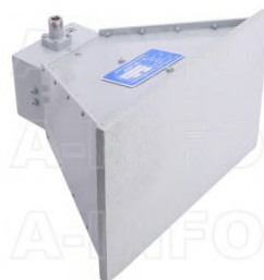
LB-1080-NFSP0 Broadband Horn Antenna 1-8GHz 11dB Gain N Type Female
