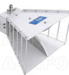
LB-7180-NF Broadband Horn Antenna 0.7-18.0 GHz 12dB Gain N Type Female
