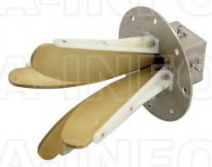
LB-OSJ-20180-SF Open Boundary Quad-Ridged Dual Polarization Horn Antenna 2-18GHz 13dB Gain SMA Female
