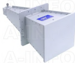
LB-20180H-NFSPPO Broadband Horn Antenna 2-18GHz 17dB Gain N Type Female
