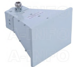
LB-20180-NFSPO Broadband Horn Antenna 2-18GHz 12dB Gain N Type Female
