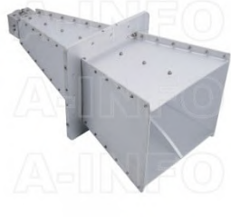
LB-20200H-SF Broadband Horn Antenna 2-20GHz 17dB Gain SMA Female
