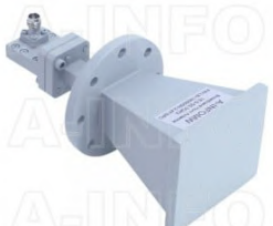
LB-180500H-2.4FSPO Broadband Horn Antenna 18-50GHz 20dB Gain 2.4mm Female
