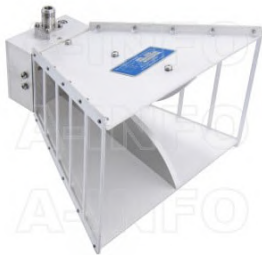
LB-7180-NF Broadband Horn Antenna 0.7-18.0 GHz 12dB Gain N Type Female
