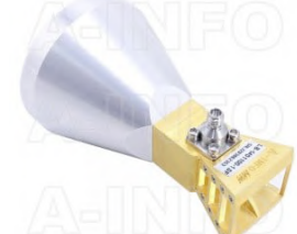
LB-1401100-1.0F Broadband Horn Antenna 14-110GHz 13dB Gain 1.0mm Female
