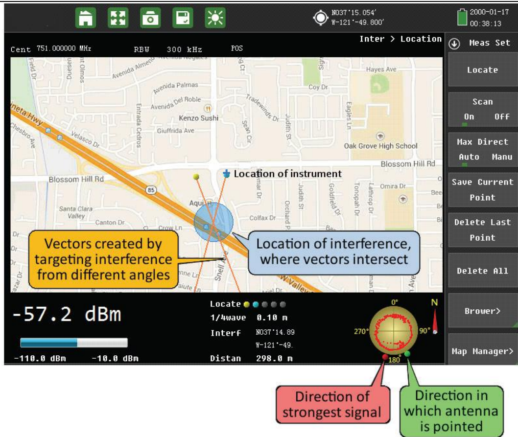
Fig.29.1 Interference mapping measurement w/two vectors
