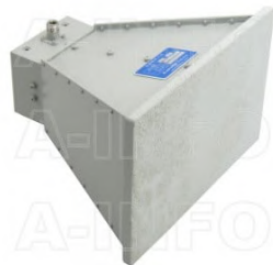
LB-880-NFSPS Broadband Horn Antenna 0.8-8GHz 10dB Gain N Type Female
