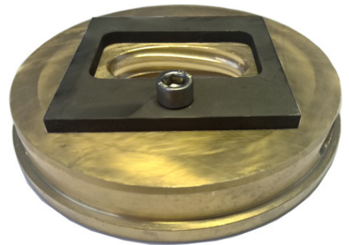
Picture shows flanging die for E65 waveguide
